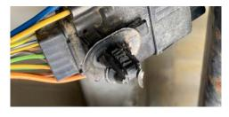
6. Using a plastic rivet removal tool, free the connector from the vehicle.
