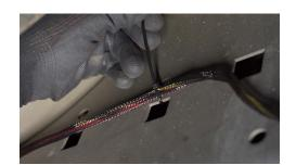
13. Route the connector end of the harness down underneath the vehicle however you see best fit. For this application, we recommend following the wheel well underneath, making sure to avoid any hot or moving parts.
