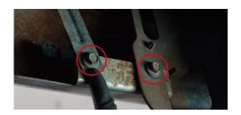
1. Using a 13mm socket and ratchet, remove the factory bolts shown in the picture above on the underside of the truck bumper.
