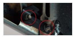
2. Install your new reverse light bracket onto the vehicle using the factory bolts removed in the previous step.
