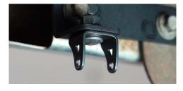
3. Install the universal pod bracket onto the reverse light bracket using the provided hardware. Make sure that the curved portion of the bracket is facing towards the rear of the vehicle.
